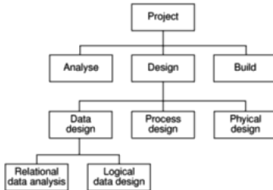
A fragment of an activity-based Work Breakdown Structure.
