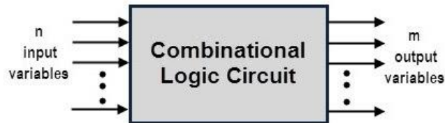
Fig: Block diagram of combinational circuit
